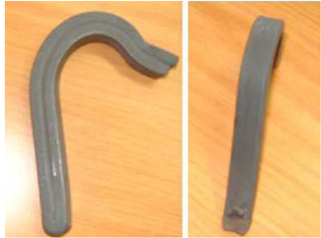
Fig. 1 Part: forged steel with tight crack
