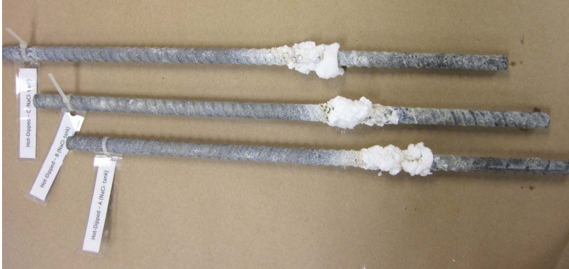
Figure 1 Traditional Hot Dipped galvanizing after 10,700 hours partial immersion
