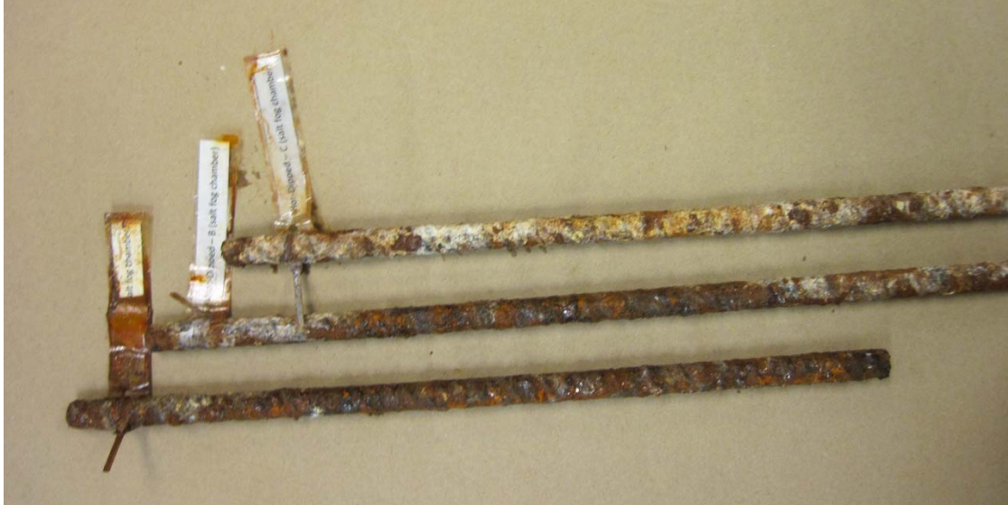
Figure 3 Traditional Hot Dipped galvanizing after 10,700 hours in salt fog exposure
