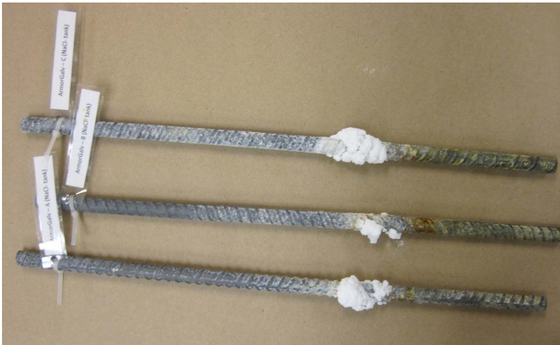
Figure 2 Armorgalv ® process after 10,700 hours of partial immersion
