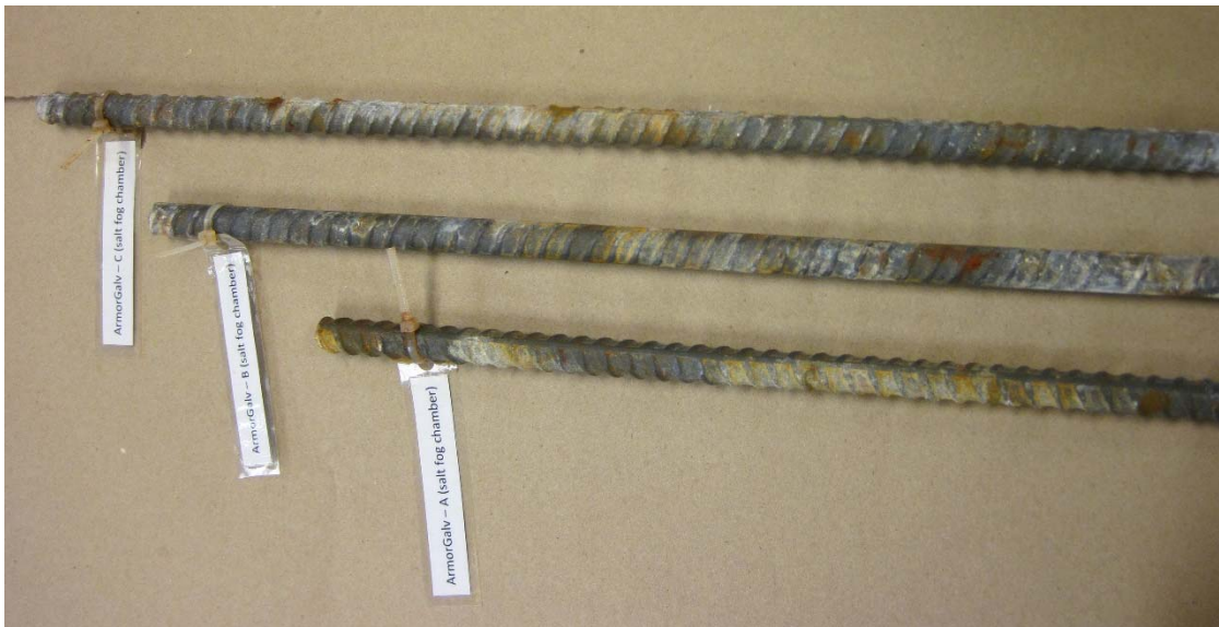
Figure 4 Armorgalv ® process after 10,700 hours in salt fog exposure
