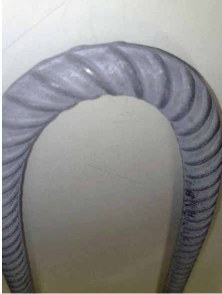
Bent rebar, coated with ArmorGalv® - No flaking or peeling.
