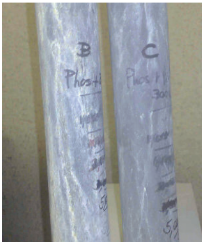
ArmorGalv® Natural 400 microns, 5000-hour B117 salt spray.
