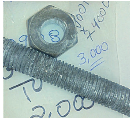
ArmorGalv® Bronze 25 microns, 4000 hr. B117 salt spray.
